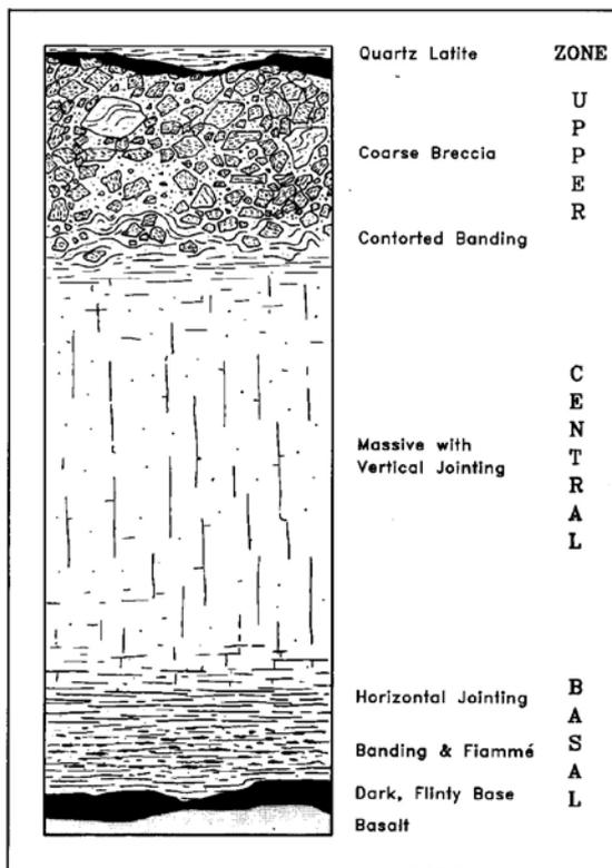
Fig. 4: A schematic section through an idealised Goboboseb quartz latite flow unit. (see Table 1a for range of typical thickness).
